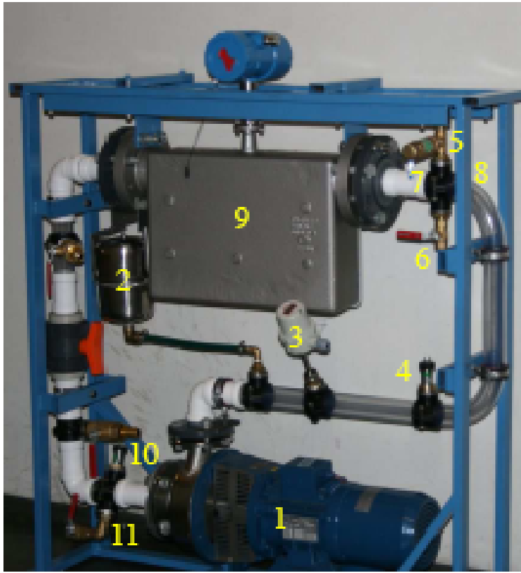
Figure 5.1: Photo of the experimental flow loop by Balakin et al. [4]. (1 - Centrifugal pump; 2 - Expansion tank; 3 - Thermocouple; 4,5 - Pressure sensors; 6 - Sampling unit; 7 - Ventilation; 8 - Safety valve; 9 - Flow meter; 10 - Pressure sensor, 11 - Drainage). Adopted by courtesy of Boris Balakin.
