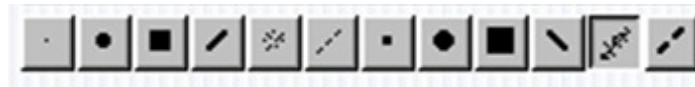
Figure 45 - Different pen splits available in VISI. The toolbar has been rotated 90 degrees.
