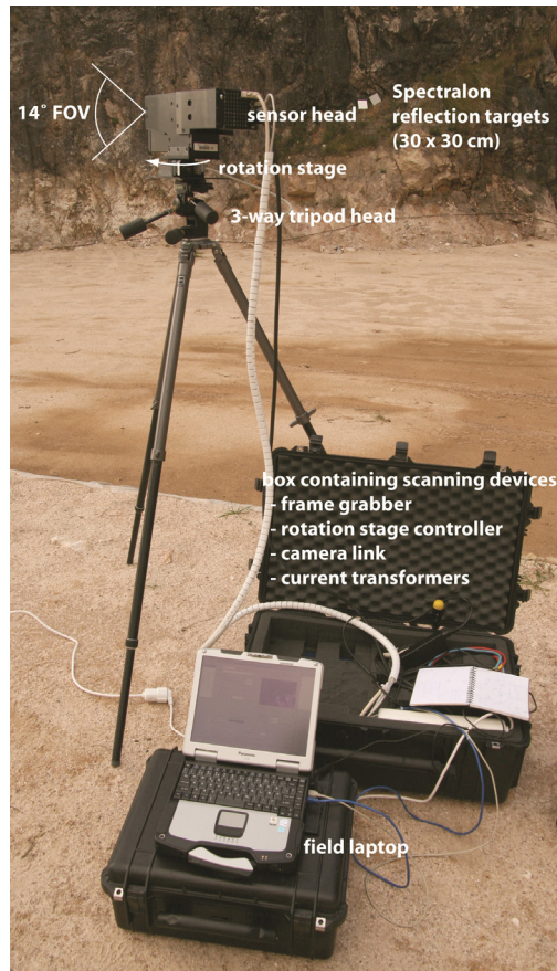
Fig 7 HySpex SWIR-320m scanning system.
