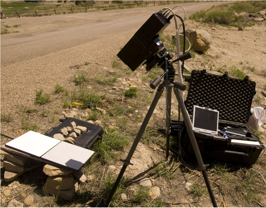
Fig 12 Scanning setup with the 1 m lens to collect rock sample spectra in the field.
