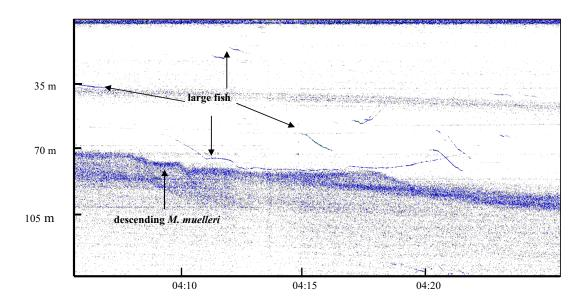
*Figure 3:* Echogram from a 38 kHZ splitbeam echosounder placed on the bottom showing migrating *M.* muelleri and several large fish tracks with a Ts between -30 and -35dB dB in Masfjorden. The distance of these acoustic targets from the echosounder is between 250 and 390 m.
