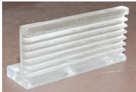
Figure 3-13: Photography of one of the slits made of Plexiglas with seven multiple crosswise grooves.
