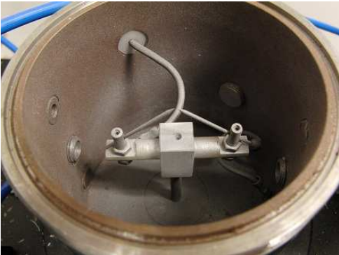
Figure 3-6 : Photography of the adjustable ignition source located in the primary chamber.
