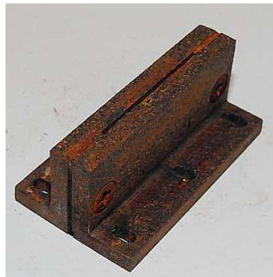
Figure 3-9: The same slit set after 3 months at sea side. Significant rust formation over the entire surface, including the flame gap surface.
