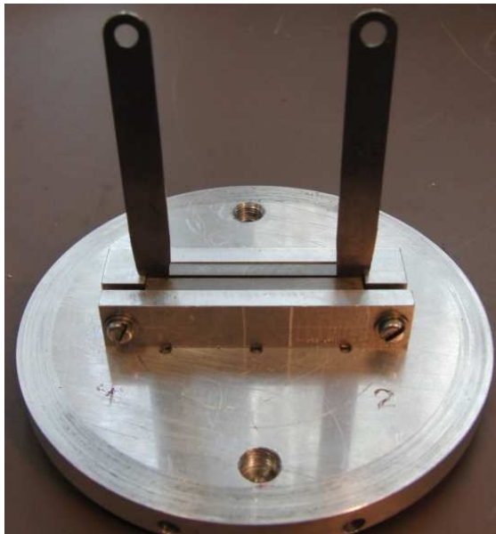
Figure- I: Photograph of the upper part of the flame gap in the PRSA, with distance "shims" placed, the gap is fastened with a small torque applied on the screws seen in the photograph
