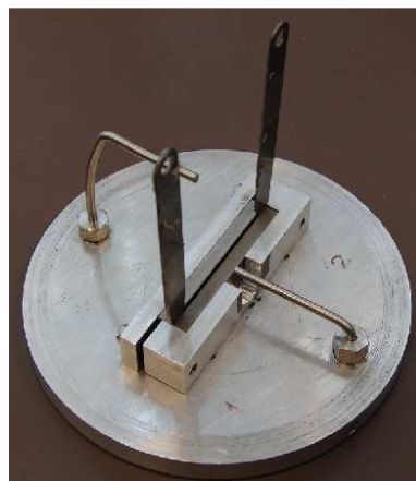
Figure 3-5: Photography of the replaceable steel rods on which the thermocouples were “clips” on.
