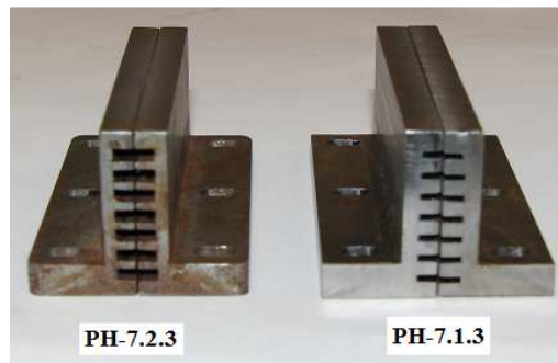
Figure 3-12: The two different slit sets with multiple crosswise grooves with different width.
