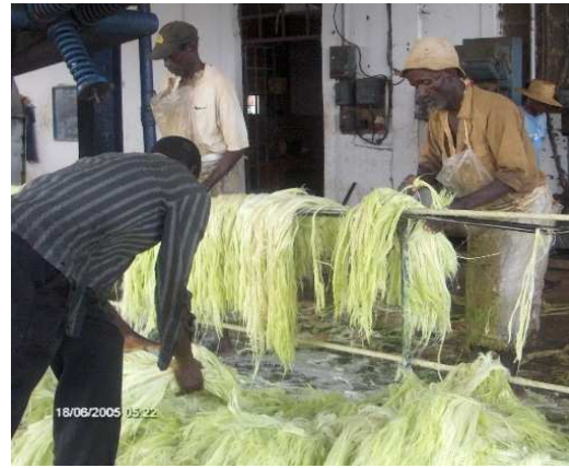
Figure 5: Tying of wet sisal fibres
