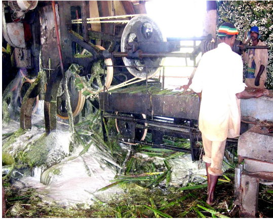
Figure 4: Decortication of sisal leaves
