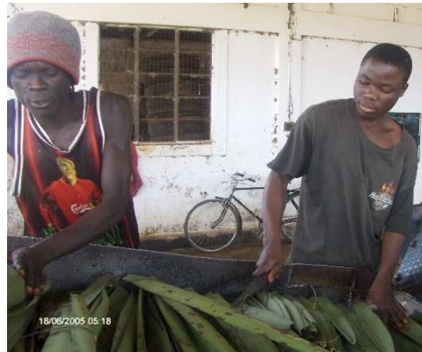
Figure 3: Feeding sisal leaves onto the conveyor
