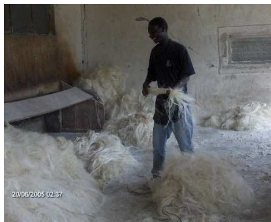
Figure 9: Re-sorting of non brushed fibres
