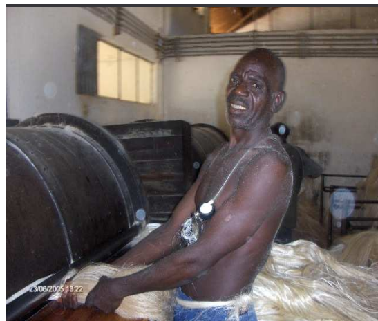
Figure 7: Brushing of sisal fibres
