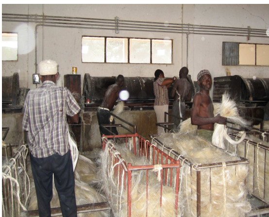
Figure 8: Sorting & grading of brushed fibres
