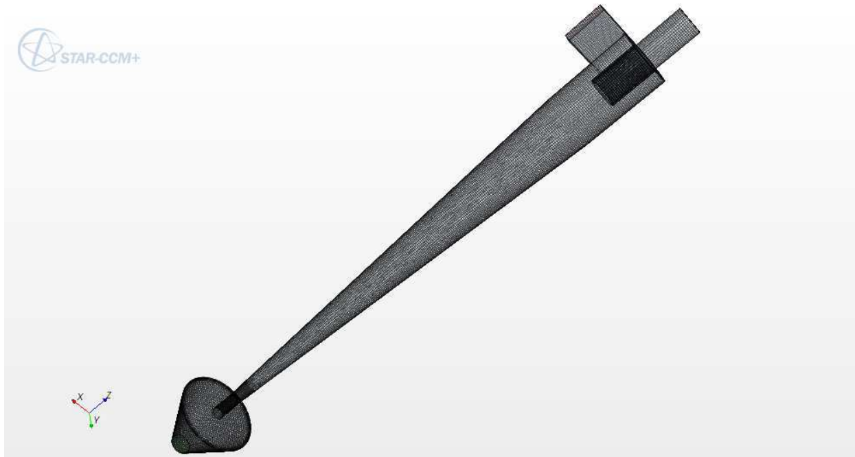
Figure 6.1: Meshed geometry used for simulations.
