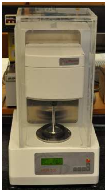
Figure 5.4: Anton Paar MCR 300 plate and cone rheometer.
