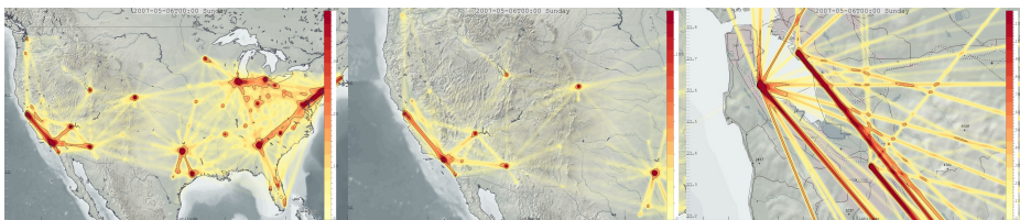
Figure 1: Interactive zooming towards SF Bay, where at first all the traffic from the Bay Area is aggregated, to a view where we can separate traffic from the three major airports, and even the distribution of traffic in each airports' cardinal direction. This interaction is enabled by automatically updating the bandwidth of the KDE when the viewport changes.
