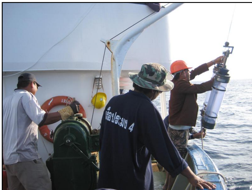
Figure 2.4 The Van Dorn 20 liters water sampler.
