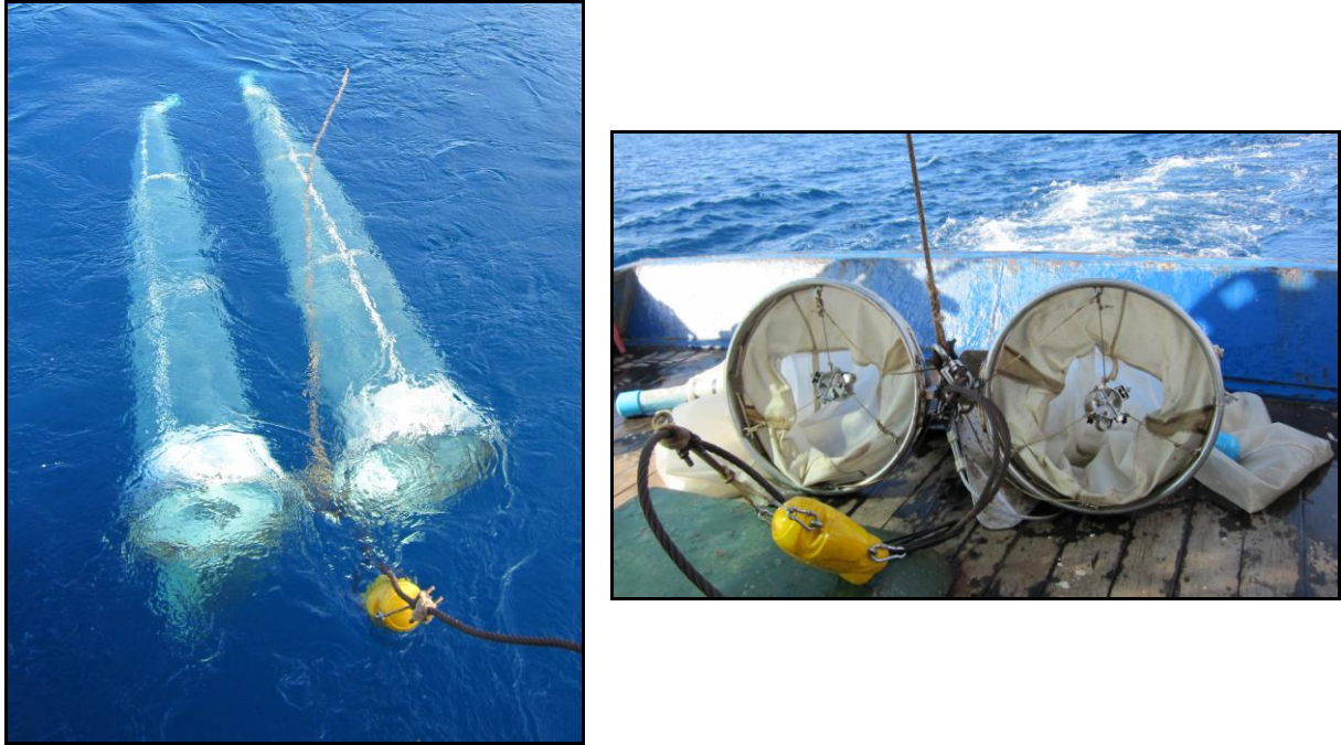
Figure 2.3 The 60 cm diameter Bongo nets during retrieval. Flow meter and depth sensor is shown in front of the nets.
