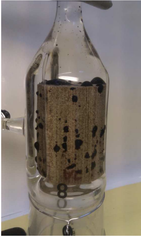
Figur 5-5: Image showing the production of oil after 5 minutes from a non-aged Berea sandstone. Since the oil clings strongly to both the core and to the glass, the imbibitions cell must be carefully “whirled” to force oil up to the graduated cylinder where it is recorded. PHOTO: Joar Vevle
