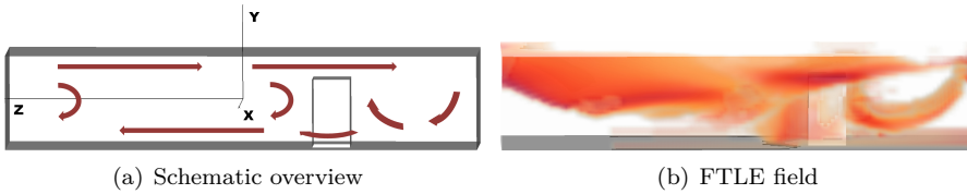
Figure 5: (a) Schematic overview over the flow domain, z being the streamwise direction. (b) The FTLE field of a simulation of a bursting dam with parameters t_0 = 62 and T = 68 . The FTLE values greater than 0.25 are brushed (smooth lower bound 0.2). We see that we can identify expected structures around the obstacle. The upper rear part of the flow domain shows large regions with high FTLE values, presumably induced by shearing.
