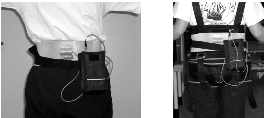
Figure 5: Person wearing a trunk accelerometer with a fixation belt and registration box (with and without wearing a harness) used in paper 1.
