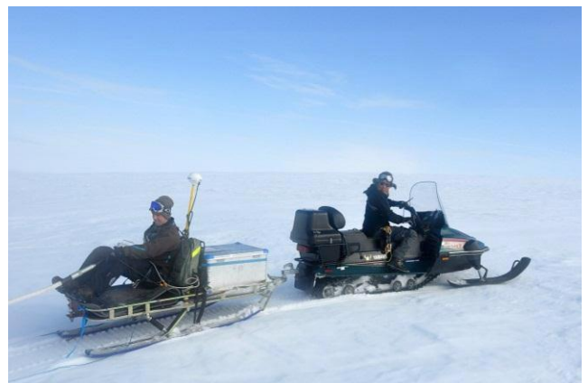
Figure 12: Collecting ice thickness measurements using Georadar equipment towed behind a Snowmobile. (Photo: Åsmund Bakke). A combination of GPR and ICE-Radar measurements were used to map the subglacial drainage of Nordfonna.
