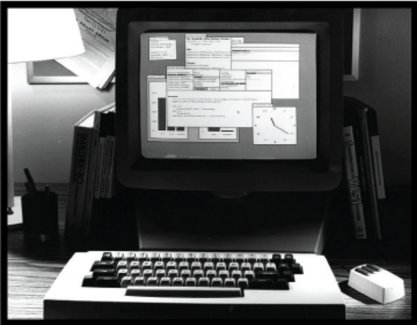
Fig. 1.10 Smalltalk environment in action on the Xerox Alto. Courtesy of Marcin Wichary via the Digibarn Computer Museum.
