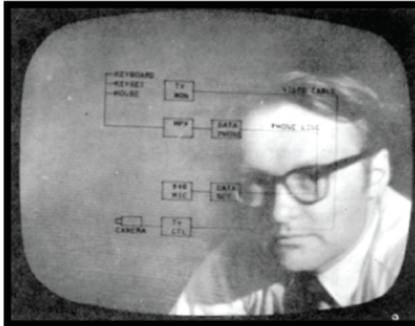
Fig. 1.9 Picture of the NLS screen presented in the article “Augmenting the Human Intellect”, with photo text: “Television display obtained by mixing the video signal from remote camera with that from the computer-generated display.”
