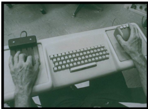
Fig. 1.8 Engelbart's control desk for the NLS, consisting of the 5 finger chord keyset, a keyboard and the 3 button mouse
