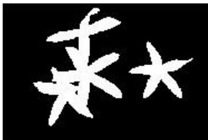
(d) Segmented result with edge detector (2.2) using \sigma = 0.8 , a = 1 , b = 30 .
