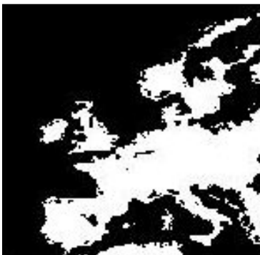
(d) Segmented result with edge detector (2.2) using \sigma = 5 , a = 0.5 , b = 1 .
