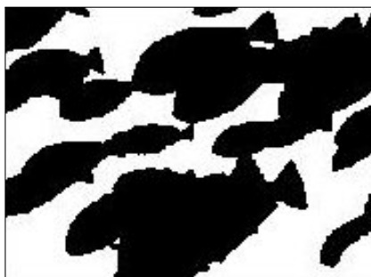
(d) Segmented result with edge detector (2.2) using \sigma = 0.5 , a = 0.5 , b = 90 .
