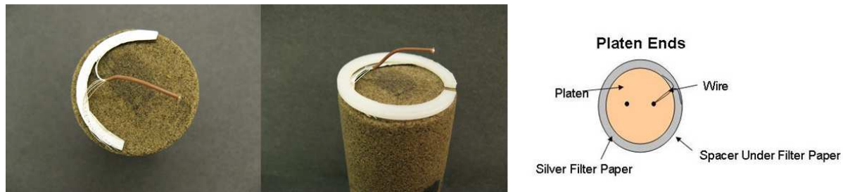
Figure 14 – Silver filter paper, contacting both trans-axial core faces, were used as electrodes in the MRI system. A POM spacer was positioned on top to provide space for the wire, which was connected to a LCR meter through a pass-through connection.
