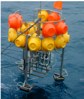
Figure 7: Benthic Chamber System (NIVA/CO 2 GeoNet)
